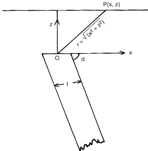
Fig. 1. Cross-sectional view of the thin dike model (2-D).
