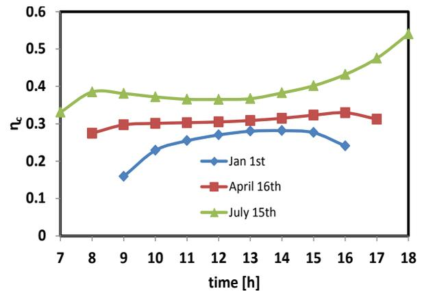
**Fig 6.** Hourly solar collector efficiency
