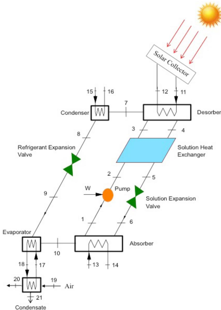
**Fig.1.** Schematic of the chiller system
