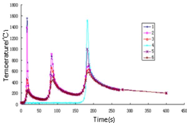
**Figure 9:** 90° Six Special Point temperature at different time step from the Weld Start
