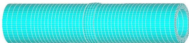
**Figure 3:** 3D Pipe Model Mesh Weld Area Enlargement
