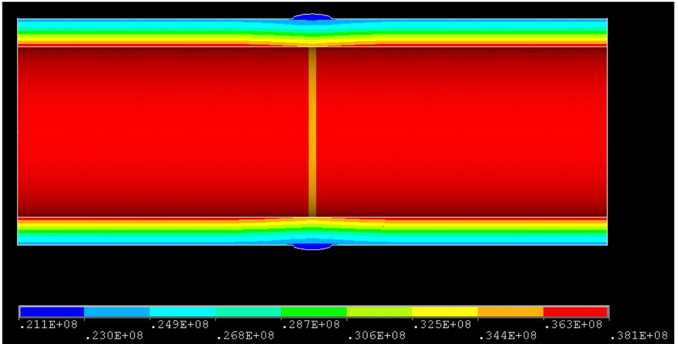
**Figure 12:** No Residual Stress Pipeline Weld Head Under 10Mpa Uniform Inner Pressure of Von Mises Stress Distribution
