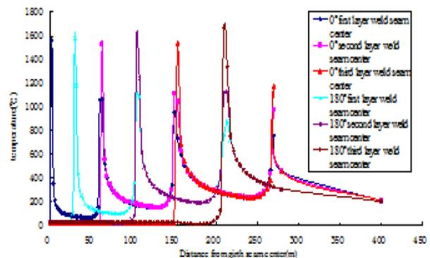
**Figure 8:** 0° and 180° Weld Seam center Temperature at Different Time Step from the Weld Start
