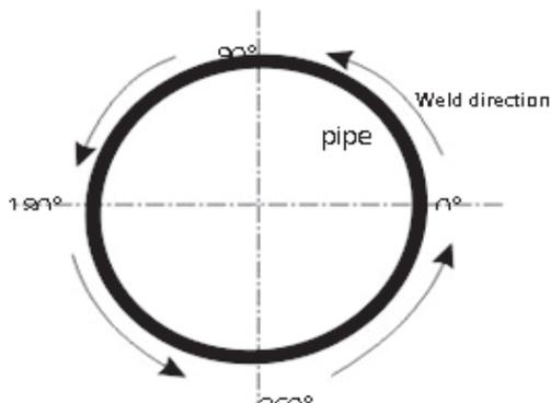
**Figure 7:** Direction of Simulative Heat Source
