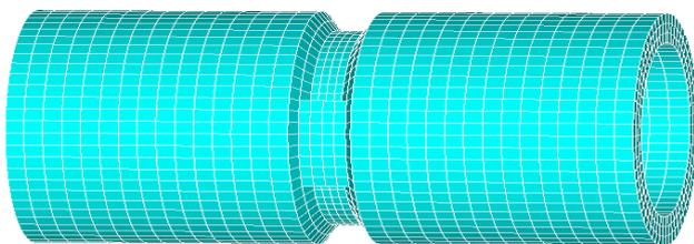
**Figure 5:** 3D Mesh Model of the Girth Weld Second Layer
