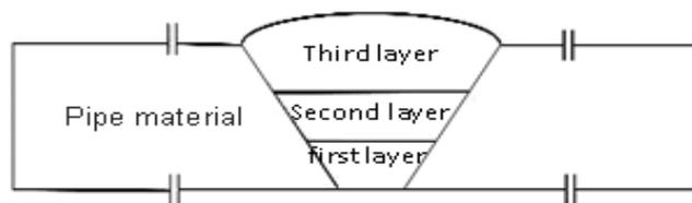
**Figure 1:** 2D Pipe Girth Weld Seam Model
