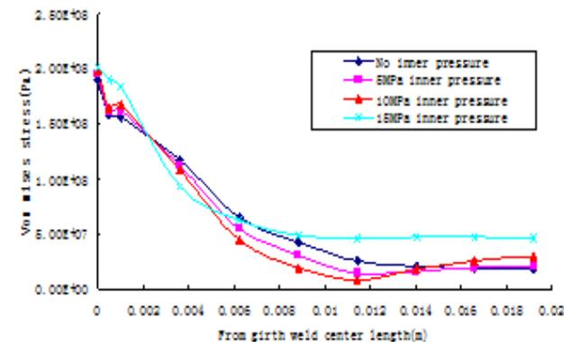
Figure 14d. The Maximum Von mises stress of Pipeline weld head third layer outer surface from the distance along the axis
