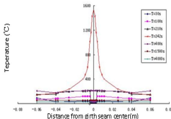
**Figure 11:** 270° Pipe Weld Head Outer Surface Axial Temperature Distribution at Different Time Step from the Weld Start
