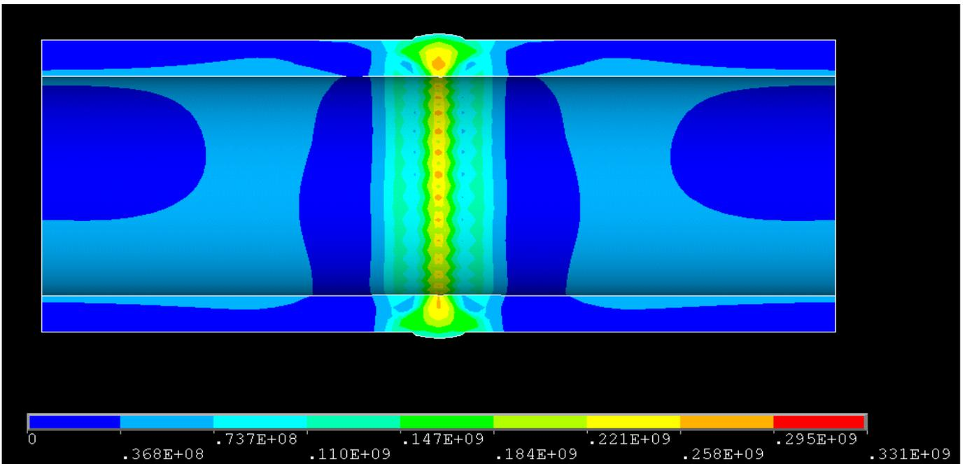
**Figure 13:** Pipeline Weld Head with Residual Stress Under 10Mpa Uniform Inner Pressure of Von Mises Stress Distribution
