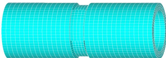
**Figure 6:** 3D Mesh Model of the Girth Weld Third Layer
