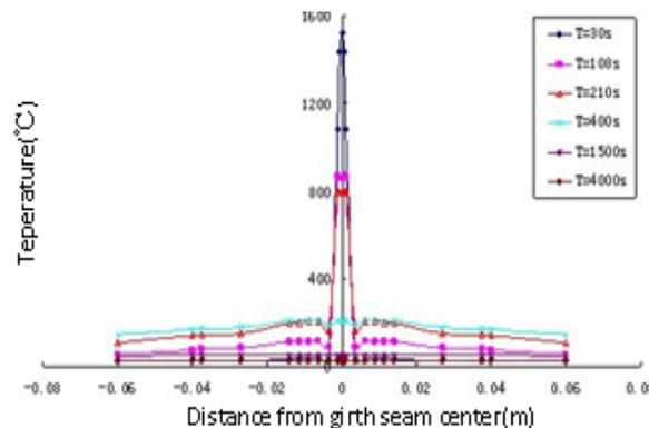
**Figure 10:** 270° Pipe Weld Head Inner Surface Axial Temperature Distribution at Different Time Step from the Weld Start
