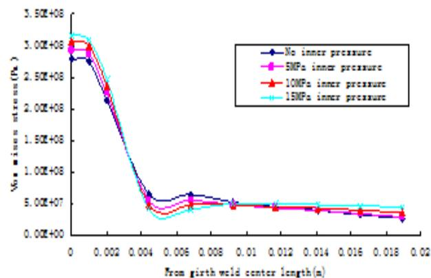
**Figure 14B:** The Maximum Von Mises Stress of Pipeline Weld Head First Layer Outer Surface from the Distance Along The Axis
