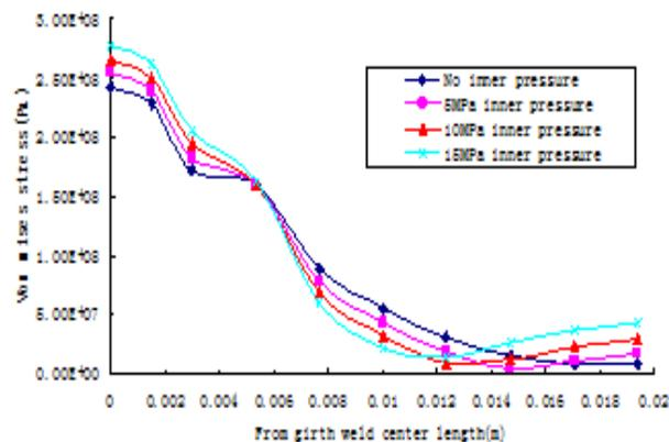
**Figure 14C:** The Maximum Von Mises Stress of Pipeline Weld Head Second Layer Outer Surface from the Distance Along The Axis
