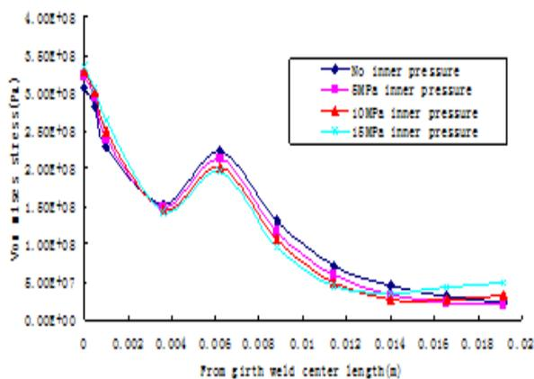
**Figure 14A:** The Maximum Von Mises Stress of Pipeline Weld Head Inner Surface from the Distance Along The Axis
