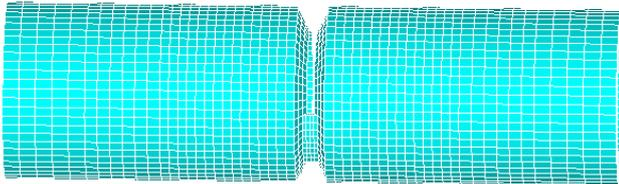
**Figure 4:** 3D Mesh Model of the Girth Weld First Layer
