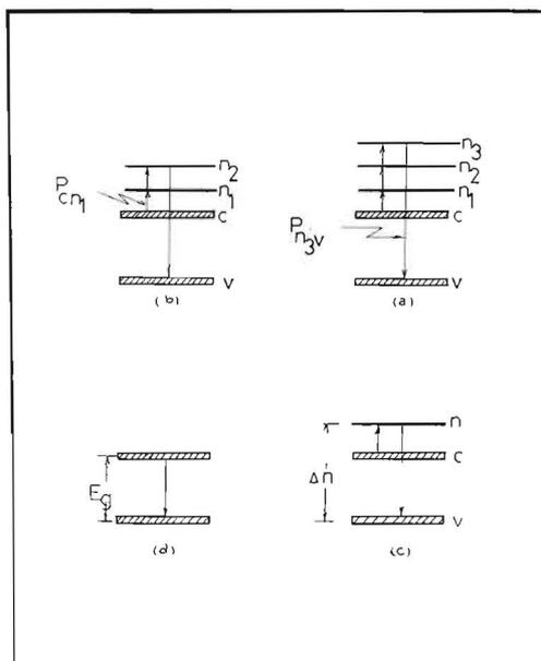
Fig. 1. A schematic diagrams representing the five- (a), four- (b), and three- (c), and two- (d) band models. The arrows indicate the coupling matrix elements.
