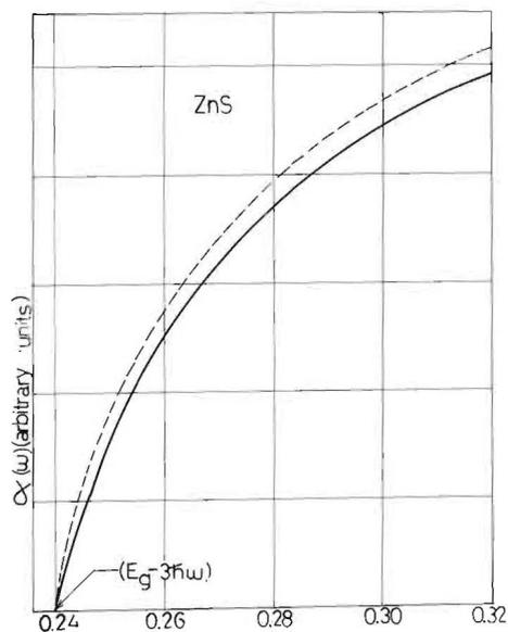
**Fig. 2.** Behaviour of the four-photon absorption coefficient as a function of the photon energy for the case of ZnS. The solid curve is the theoretical calculation and the dashed curve is the experimental data by Catalano *et al.* (1975).
