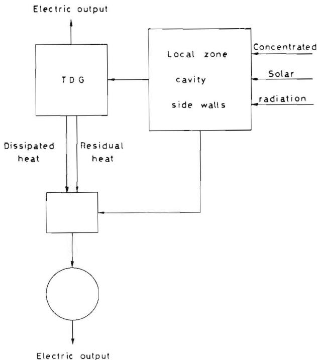
Fig. 4. Block diagram illustrating heat transfer in the CTR.
