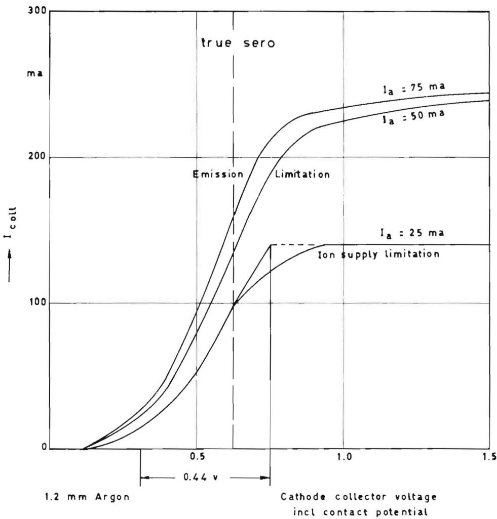
**Fig. 1.** Characteristics of the simple experimental tube shown in Fig. 2.
