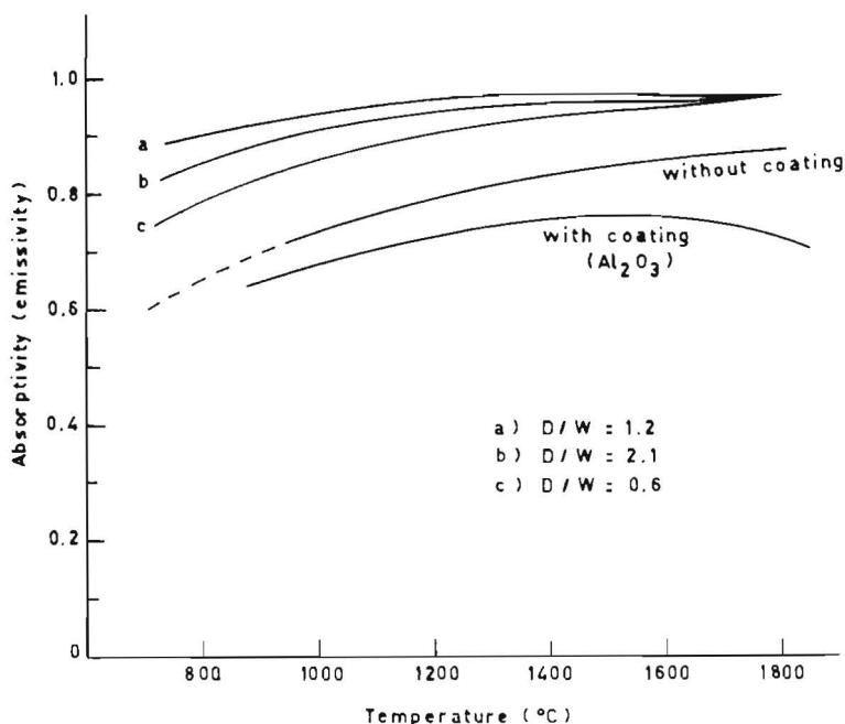
**Fig. 5.** Absorptivity of silicon carbide in the region of  $0.5 \mu\text{m}$  (maximum of solar radiation).
