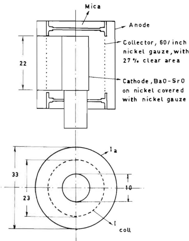
Fig. 2. Thermionic diode configuration.
