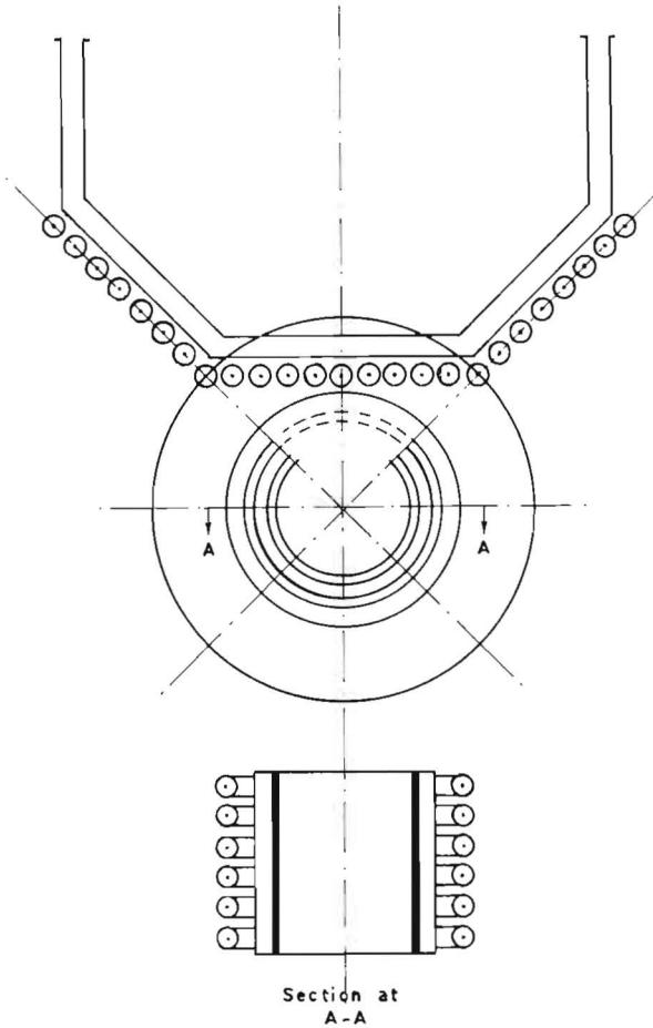
Fig. 3. Cavity heated air central receiver.
