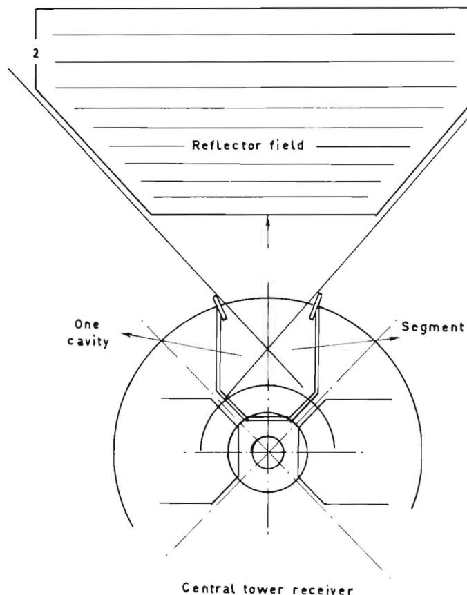
Fig. 6. Cavity shape and field of view of the receiver focal zone.
