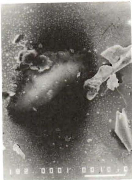
**Plate 3.** SEM micrograph showing the pit and its surroundings in a glass substrate coated by a nickel film.
