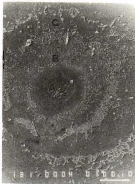
**Plate 1.** SEM micrograph of the pit in a damaged glass substrate coated by an antimony film.
