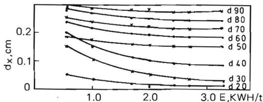
Fig. 4. The relation between ( $d_x$ ) and energy ( $E$ ) for an initial size of  $S_i = 0.283$  cm.
