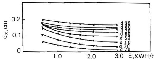
Fig. 6. The relation between ( $d_x$ ) and energy ( $E$ ) for an initial size of  $S_i = 0.180$  cm.
