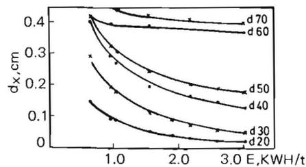
Fig. 1. The relation between ( $d_x$ ) and energy ( $E$ ) for initial size  $S_i = 0.565$  cm.
