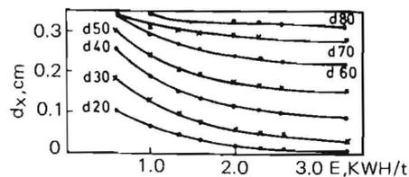
Fig. 3. The relation between ( $d_x$ ) and energy ( $E$ ) for an initial size of  $S_i = 0.358$  cm.
