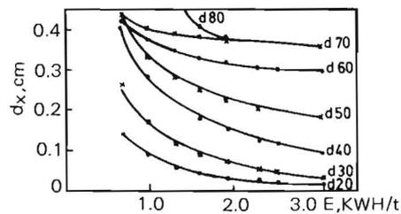
Fig. 2. The relation between ( $d_x$ ) and energy ( $E$ ) for an initial size of  $S_i = 0.45$  cm.
