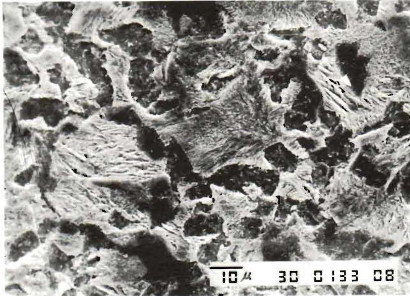
Fig. 1. Pearlite and proeutectoid ferrite in the as received steel.
