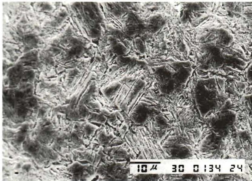
Fig. 6. Showing lower and upper bainite in a palm-oil quenched specimen
