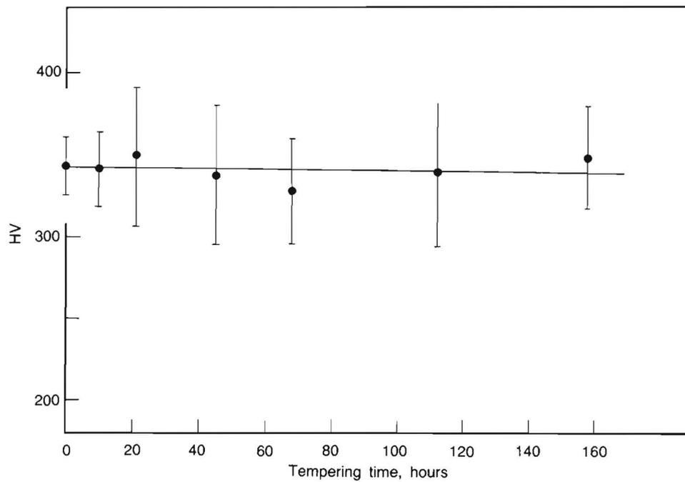
Fig. 8. Effect of tempering time at 195°C on the hardness of a Petromin-oil quenched specimen
