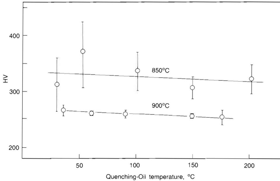
Fig. 5. Effect of palm-oil quenching temperature on the hardness of the steel
