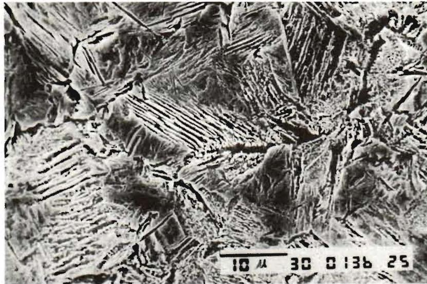
Fig. 7. Lamellar martensite formed in a Petromin-oil quenched specimen
