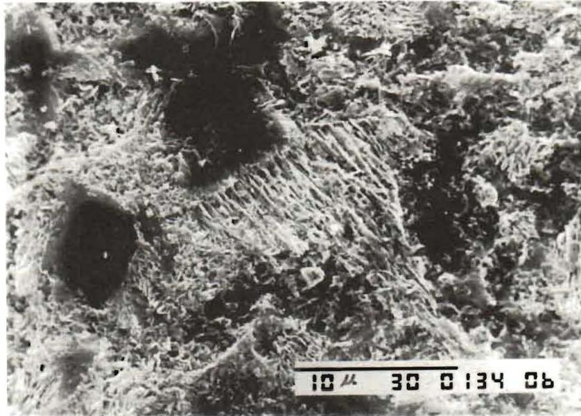
Fig. 4. The microstructure of an air-quenched specimen, showing pearlite and proeutectoid ferrite areas
