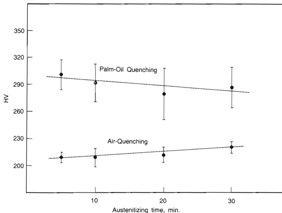
Fig. 3. Vickers hardness versus austenitizing time at 850°C
