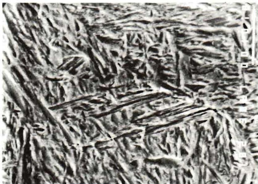
Fig. 2. Lenticular martensite structure in a water-quenched specimen.
