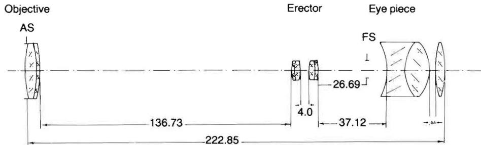
Fig. 4. The optical layout of the first telescope
