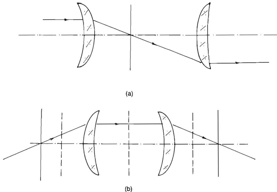
Fig. 1. Hard way and easy way couplings of modules
