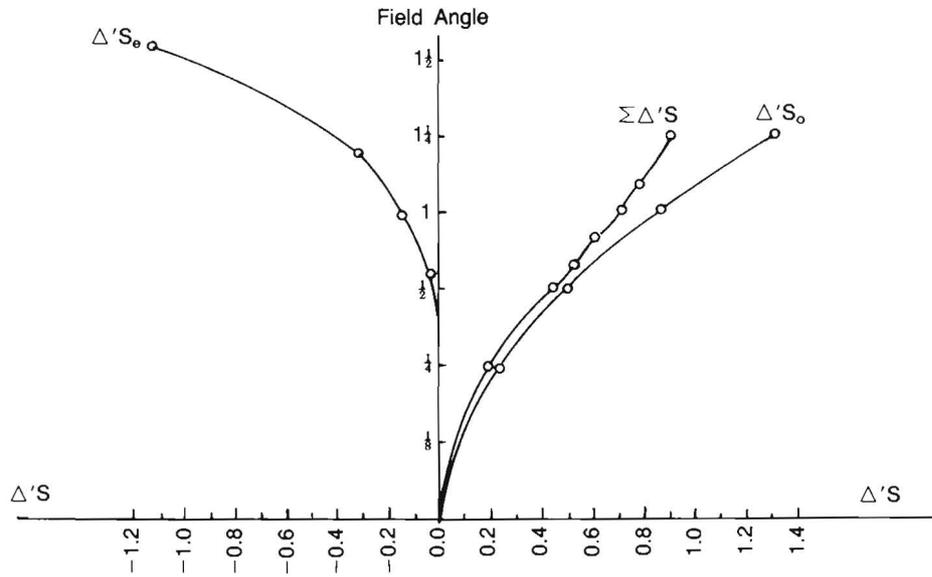
Fig. 2.  $\Delta'S$  for objective and eyepiece and for the whole system against the field angle
