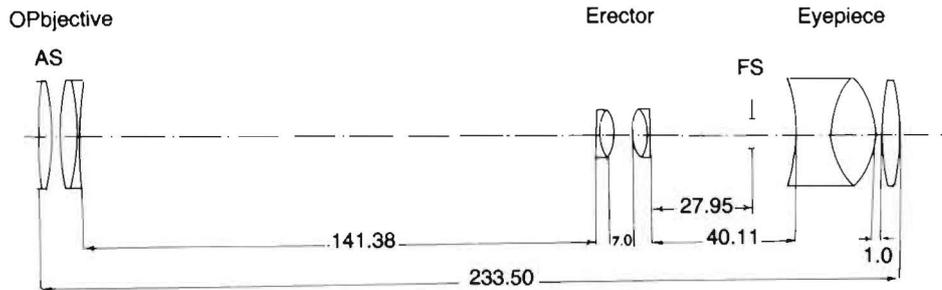
Fig. 7. The optical layout of the second telescope
