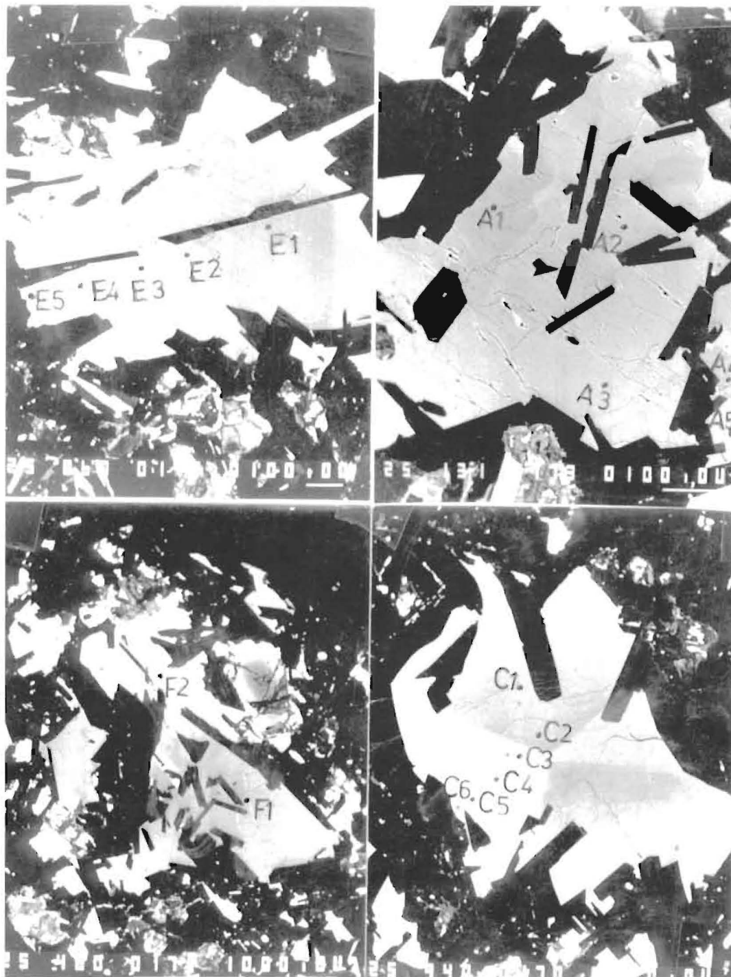
Fig. 2: Compositional type back scattered electron images of the clinopyroxenes. a) Zoned diopside megacryst in olivine basalt, b) Cryptic zoned megacryst of diopside in olivine-rich dolerite, c) Cryptic zoned groundmass grain of hedenbergite, d) Sector zoned megacryst with augitic core and hedenbergitic rim in olivine dolerite.
