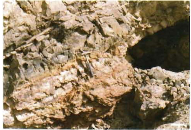
Fig. 1: Alteration zones surrounding auriferous quartz vein. Um Balad gold prospect. depleted, transitional and anomalous zones in any lateral section of alteration zone surrounding an auriferous quartz vein.
